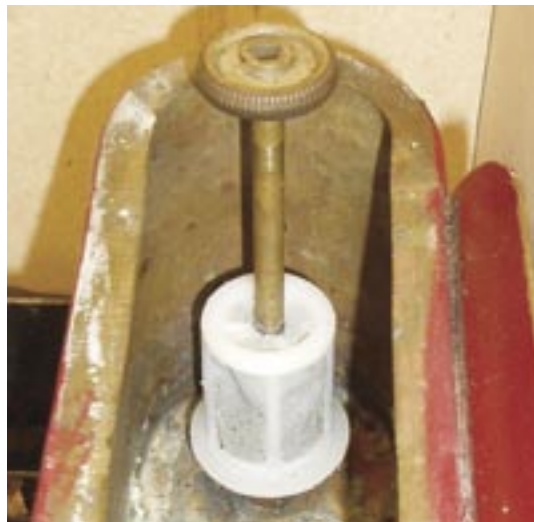
Above left: Dave's tender before fitting the filter. Above right: With the filter fitted. Left: The filter fitted to the injector water valve
