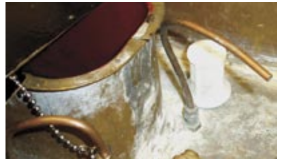
Above left: Dave's tender before fitting the filter. Above right: With the filter fitted. Left: The filter fitted to the injector water valve
